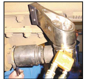
Patented Multi-Axis Swivel provides for better accessibility and prevents hose kinking.
